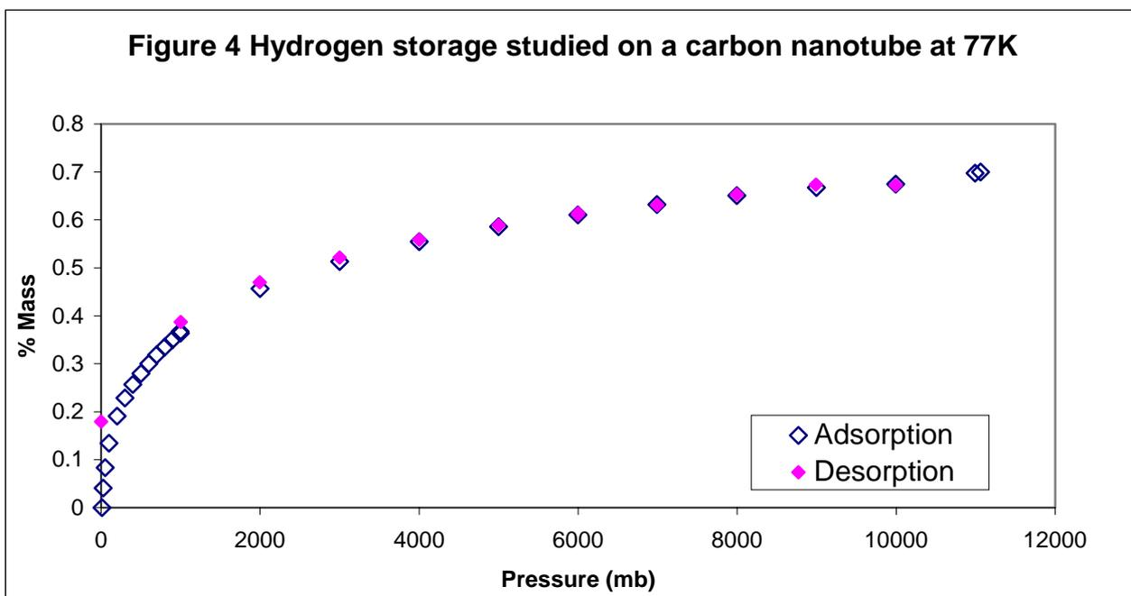
Figure 4 is an example of an hydrogen absorption/desorption isotherm measured using the
